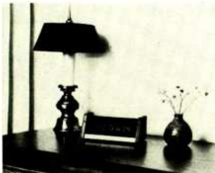
FIG. 1—THE 6-DIGIT DESK CLOCK with Numitron display blends into almost any home or office decor. Smoke-gray or clear "see through" acrylic may be used for the cover. Oiled walnut is used for the side pieces.
