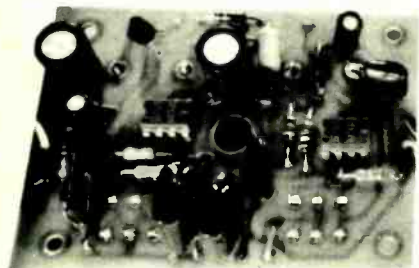
CIRCUIT BOARD of the Alpha Brainwave Monitor with all the components installed.
